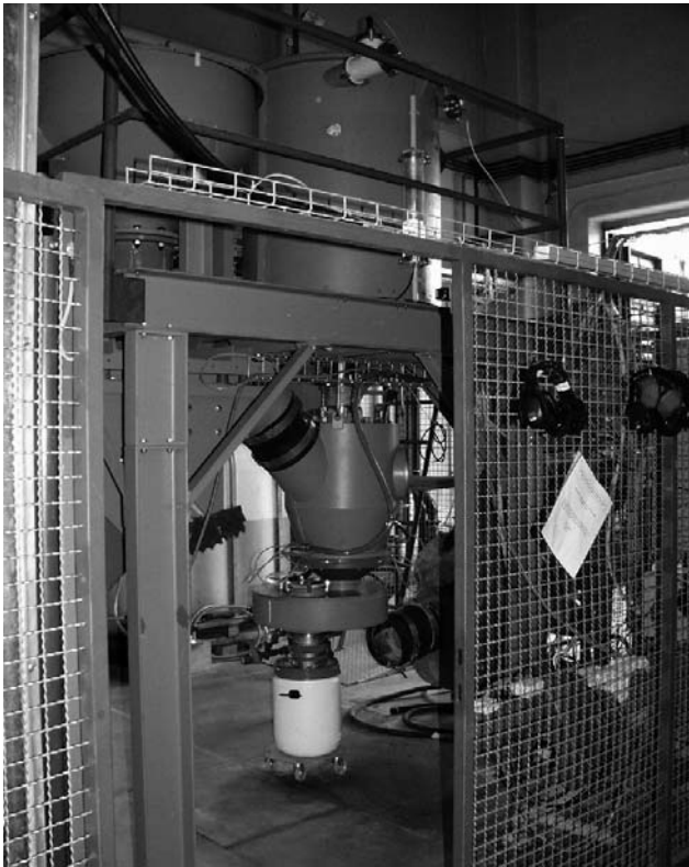
Fig. 12.11. View of FRANKA-Stein, a semi-industrial prototype to demonstrate concrete recycling with complete separation of the aggregate at a throughput of up to 1 t/h. The Marx generator is housed in the top cylindrical case
