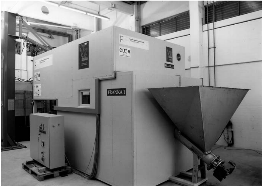
Fig. 12.12. FRANKA-1 before shipment to an incineration plant. FRANKA-1 is used to separate metallic components from the ash and to immobilise heavy metals in the ash
