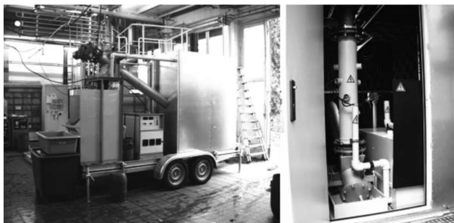
Fig. 10.5. View of the KEA mobile electroporation device. Left photograph: Faraday cage housing the Marx generator and the process chamber ( right ); power supply and screw conveyor ( middle ); and tub for collection of treated beets ( left ). Right photograph: process chamber, consisting of a polypropylene tube with four pairs of distributed electrodes
