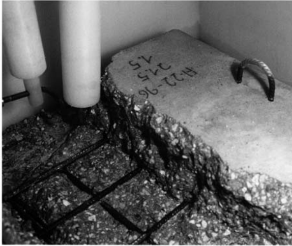
Fig. 12.15. View of a block of reinforced concrete with the surface layer removed. Here the two-electrode system shown in the upper left corner of the photograph was used
