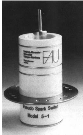
Fig. 4.18. General view of a metal–ceramic pseudospark switch
