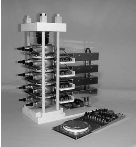
Fig. 4.29. Four-stage repetitive thyristor switch with integrated free-running diode and trigger circuit. Maximum operating voltage, 10 kV; peak current, 30 kA; maximum current rise, 20 kA/ \mu s; repetition rate, 10–50 Hz. Water-cooling bodies are visible between the thyristor units. A single unit with a trigger circuit but without water cooling is shown at the bottom .
