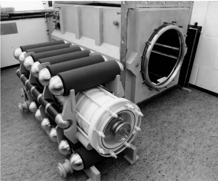
Fig. 12.8. Photograph of a 400 kV, 1.8 kJ Marx generator designed to operate at 10 Hz with a component lifetime of 10^8 pulses. The generator discharge period is 2.5 \mu\text{s}
