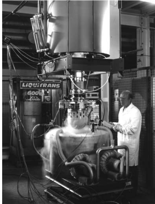
Fig. 12.18. FRANKA-3, built to explore the applicability of electrodynamic fragmentation under liquid nitrogen. The Marx generator is located in the barrel hanging from the roof
